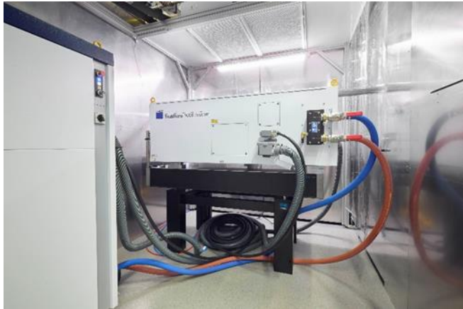
Image 3: TRUMPF TruMicro 9000: The world's first industrial 1kW-USP laser is located in the user facility of the Fraunhofer Cluster of Excellence Advanced Photon Sources CAPS at Fraunhofer ILT in Aachen. © Fraunhofer ILT, Aachen, Germany / Ralf Baumgarten.
