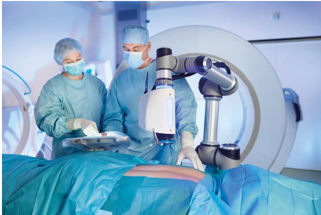
Image 1: Surgically opening the vertebral body is highly risky due to the spinal cord lying in the spinal canal. The robotically assisted laser surgery system developed at the Fraunhofer ILT is intended to replace mechanical high-speed milling and minimize surgical risks.
