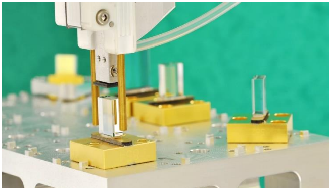
Image 4: Solder-based assembly of optics for long-term stable beam shaping. The adjustment of micro-optics is to be accelerated in the future with AI to achieve the quantities and lower the unit costs required for commercial power plants. © Fraunhofer ILT, Aachen, Germany.
