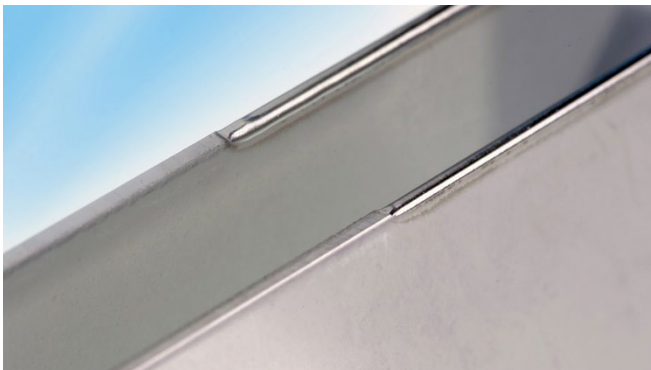
Picture 2: Partially laser-rounded stainless steel sheet edges with a sheet thickness of 1.5 mm. © Fraunhofer ILT, Aachen, Germany.
