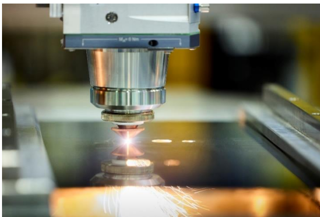
Figure 1: As part of the DIPOOL project, Dr. Frank Schneider and his team are using AI and minimally invasive laser modulation (MILM) to optimize process monitoring and control in sheet metal processing. Fraunhofer ILT, Aachen / Ralf Baumgarten.
