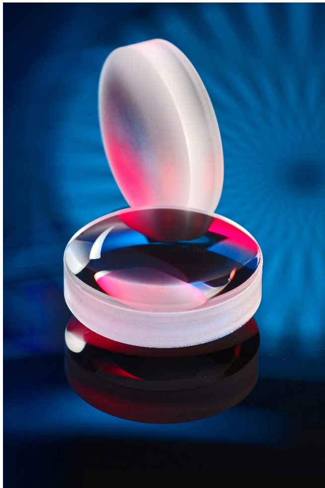
Image 1: The light scatters on the surface of the polished asphere at the back. The same optics can be seen in the laser-polished state at the front. © Fraunhofer ILT, Aachen, Germany.
