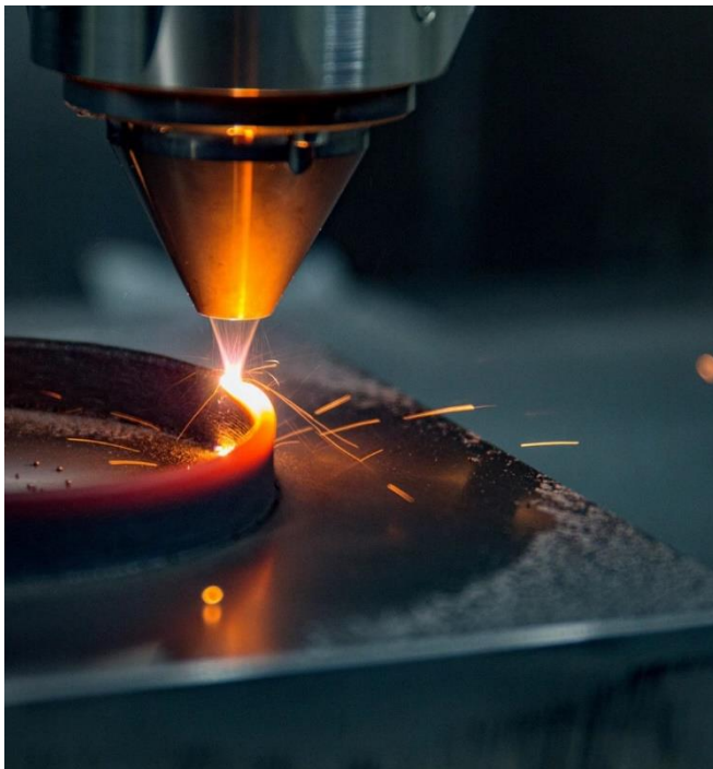
Image 2: The new production process with EHLA3D technology makes it possible to efficiently produce, coat or repair complex geometries with high-strength materials. © Makino.
