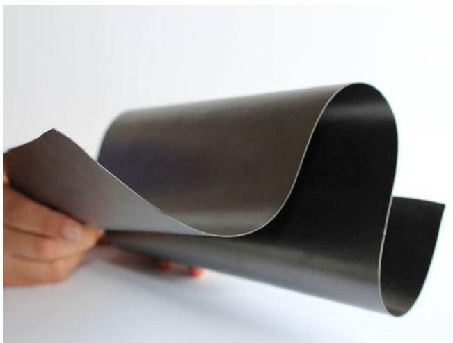
Image 1: Compound film for bipolar plates: In the HyCoFC research project, researchers are working on durable, cost-effective and powerful fuel cells for heavy-duty applications. Innovative material combinations and state-of-the-art laser technologies are being used. © Fraunhofer UMSICHT
